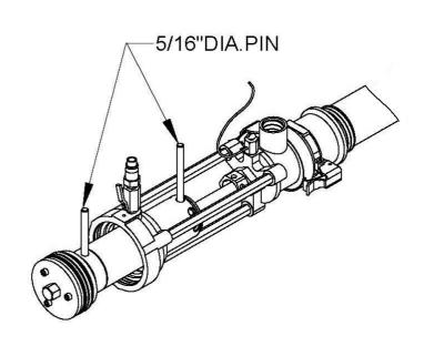
6. Remove the dowel pin from the plunger top. Air motor assembly can now be removed from the displacement plunger and main shaft.
