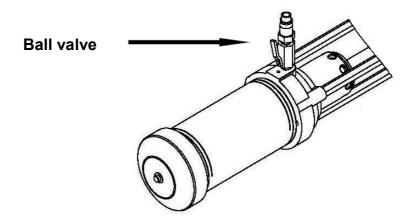
4. Place a strap wrench around the lower end of the air cylinder and carefully unthread.
