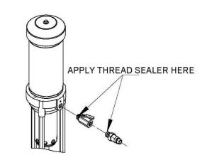
2. Screw the bung adaptor onto the mount bracket. Carefully slide the transfer pump through the adaptor and lock it in place with the bung adaptor latch hooks.
