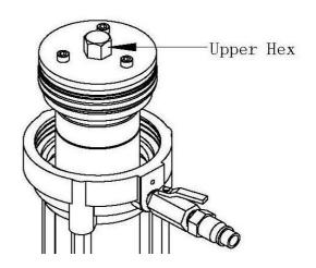
7. Remove the foot valve from the suction tube and push the main shaft out through the suction tube.
