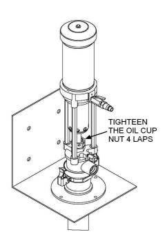
3. Attach air line onto quick disconnect fitting to complete installation. It is recommended to use a minimum 3/8" hose for the pump air supply.
