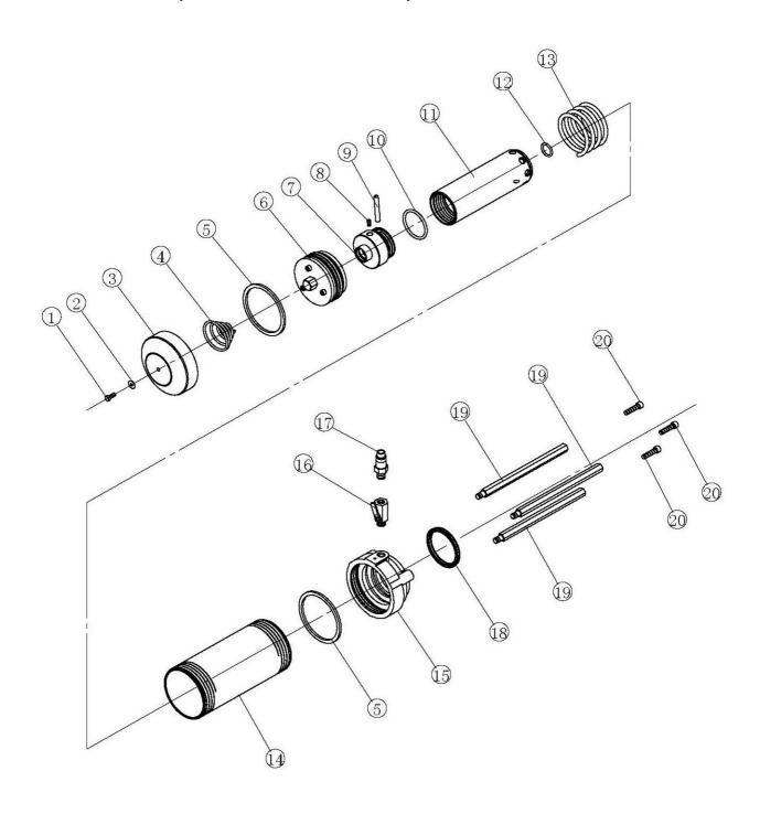
**NOTE:**When replacing Socket Set Screw (8) and the Plunger Top (7),it is important that a Liquid Thread Sealing Compound be use to prevent the assembly from vibrating loose.
